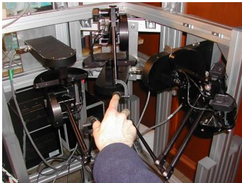
Figure 5.1: The three finger Phantom configuration used for conducting this research. This setup was chosen as it maximises the available workspace for translations and rotations of virtual objects without the mechanical arms colliding. This is the right hand setup.
