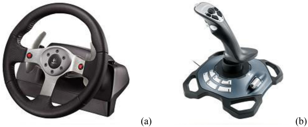
Figure 2.14: a) The Logitech G25 force feedback steering wheel uses two motors to provide the force feedback. This enables the G25 to provide the strongest force feedback possible without the problems of overheating. b) The Logitech Force ™ 3D Pro force feedback joystick [wwwLogitechGames07].
