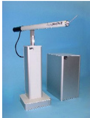
Figure 2.10: The Haptic Master produced by FCS [wwwFCS05]. Because of its size a force sensor is embedded at the endpoint that controls the direction of movement whilst in freespace.
