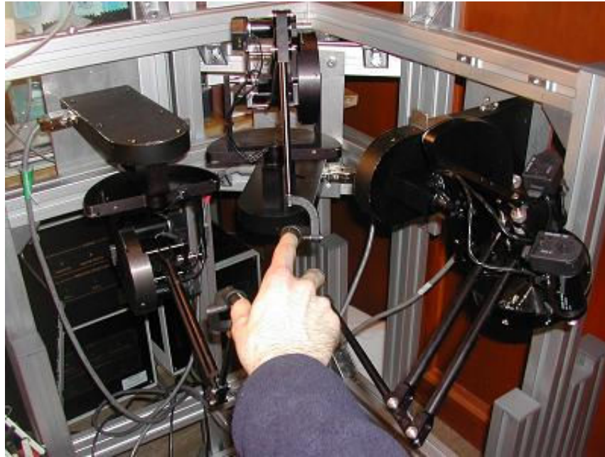
Figure 2.19: Three Phantom haptic devices mounted so that three fingers can be used to interact with the virtual world. By replacing the rightmost Phantom with a palm attachment, power grips can also be modelled. Unlike the immersion Cyber Grasp, this setup is fully grounded and so allows for the simulation of weight as well as shape.
